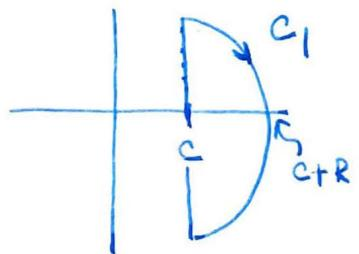
$$\oint_{C_1} F(s) e^{xs} ds = 0 \quad [\because \text{there are no singularities of } F(s) \text{ inside } C_1]$$
