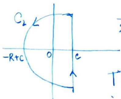
$$\frac{1}{2\pi i} \oint_{C_2} F(s) e^{xs} ds = \frac{1}{2\pi i} \times 2\pi i \times (\text{Residue at } s=0)$$
