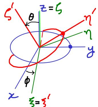
③ Rotate around  $\zeta'$ -axis (new  $z$ -axis) by  $\psi$ .
